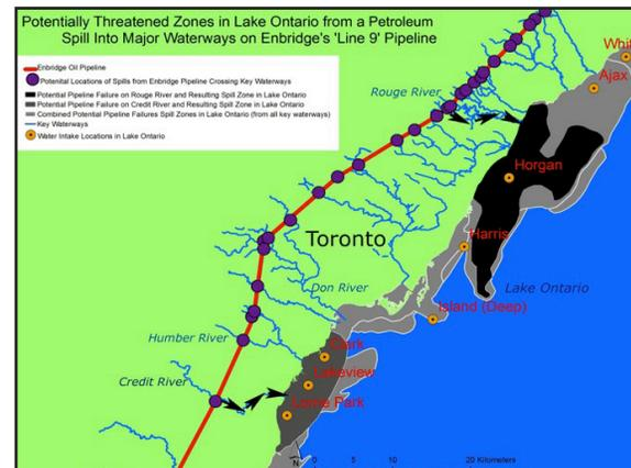
This diagram shows the effect of an oil spill into Lake Ontario, and locations of water intakes.
